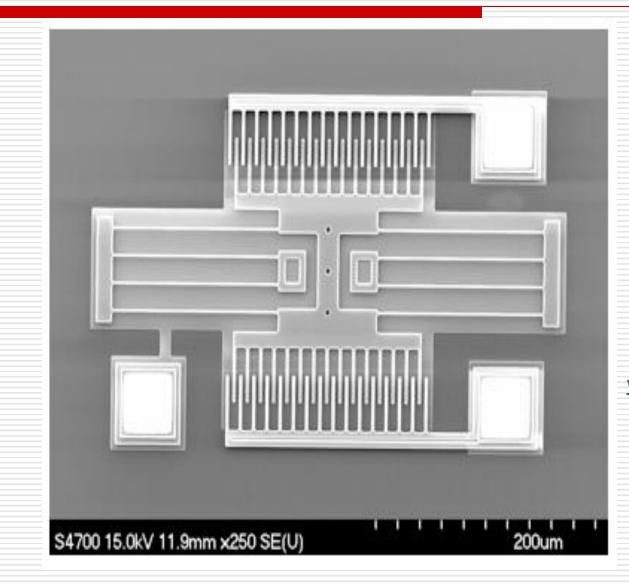
Resonator fabricated by the MNX (Can be used both as a micro-sensor and as a micro-actuator)
