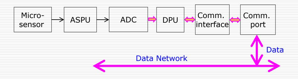
Output data of a network sensor is available on an integrated communication port in an appropriate format, which allows networking of such sensors without requiring any further interface circuitry or data formatting.
