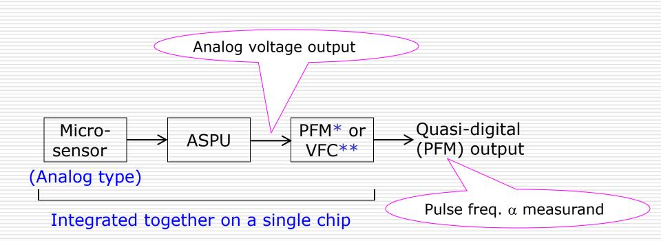
\* Pulse frequency modulator circuit
