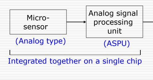
Analog output signal *DC voltage*  $\alpha$  measurand *e.g.* 0-1 V 0-2 V 0-5 V *DC current*  $\alpha$  measurand *e.g.* 0-100  $\mu$ A 0-1000  $\mu$ A
