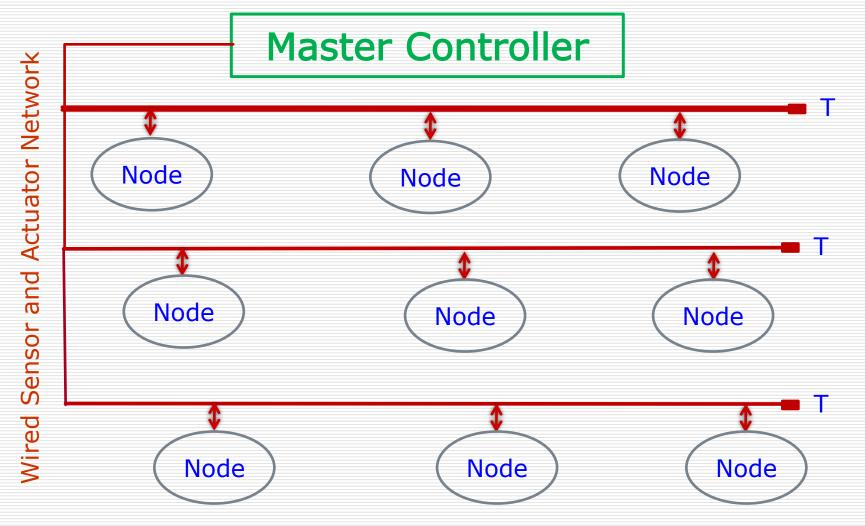
Each Node is either a 'Measuring Instrument' or a 'Control Unit'
