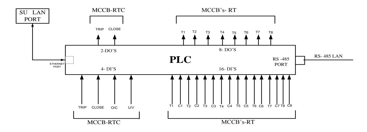
Legend MCCB-RTC: MCCB with Remote Trip & Close. MCCB-RT: MCCB with Remote Trip only. Smart Power Grid and Micro-Grid Prof. H.K
