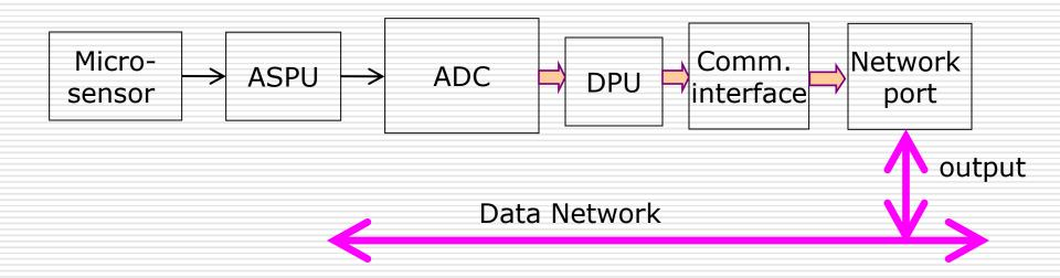
Output of a network sensor is the processed data available on an integrated network port, which allows networking of such smart sensors without requiring any further interface circuitry or data manipulation.
