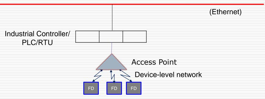
FD: Field Device (Sensor / Actuator/etc.)
